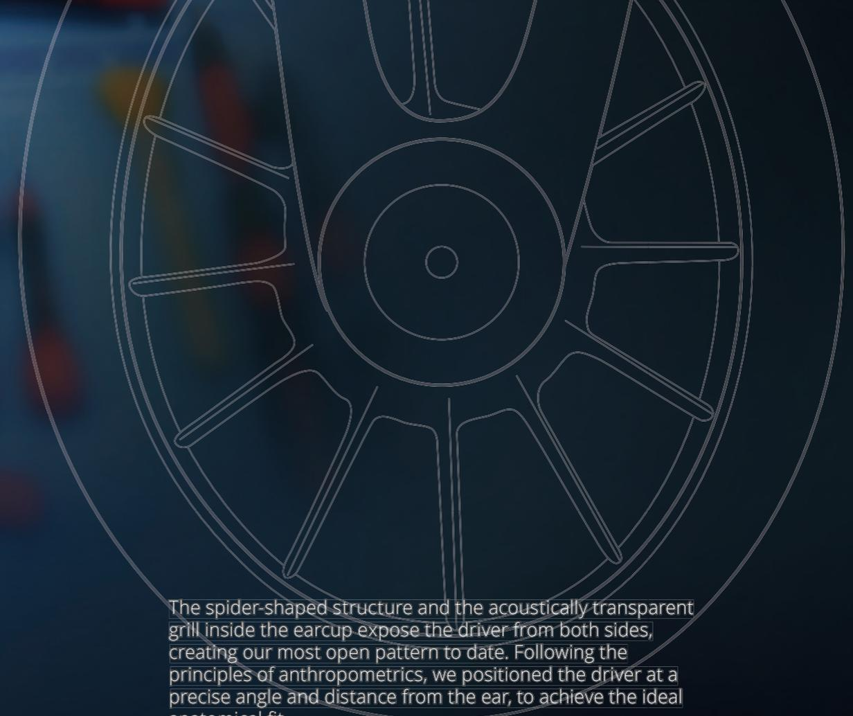
The spider-shaped structure and the acoustically transparent grill inside the earcup expose the driver from both sides, creating our most open pattern to date. Following the principles of anthropometrics, we positioned the driver at a precise angle and distance from the ear, to achieve the ideal anatomical fit.
